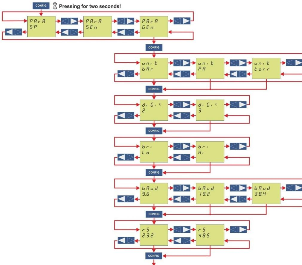
Figure 32 – Setting of the Parameter Gen
