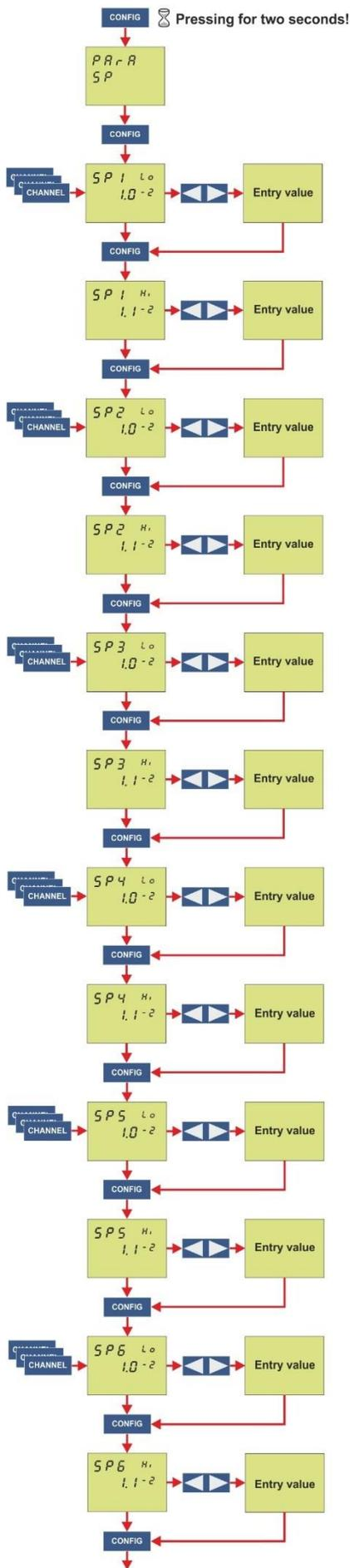
Figure 30 – Adjustment of Parameters SP
