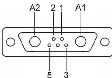
Figure 12 – Connection BA sensor (SUB-D mixed, 5-pole +2)
