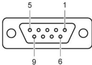
Figure 20 – Socket Interface (D-SUB, 9-pole)
