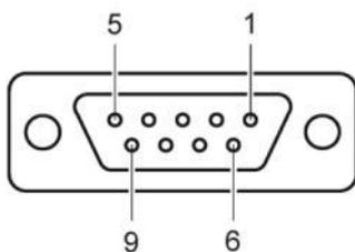
Figure 15 – Socket Interface (D-SUB, 9-pole)
