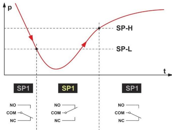
Figure 29 – Behaviour of a Switching Function in Response to Pressure Changes
