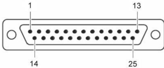
Figure 16 – Connector for Relay Output (D-SUB, 25-pole)
