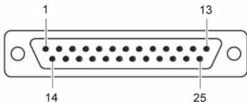
Figure 21 – Connector for Relay Output (SUB-D, 25-pole)
