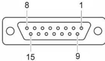
Figure 11 – Connection wide-range vacuum gauge ATMION® (D-SUB, 15-pole)
